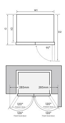
When positioned in a corner area, spacing of at least 285mm on the hinge side will allow the doors to open enough to enable the removal of bins and shelves.
