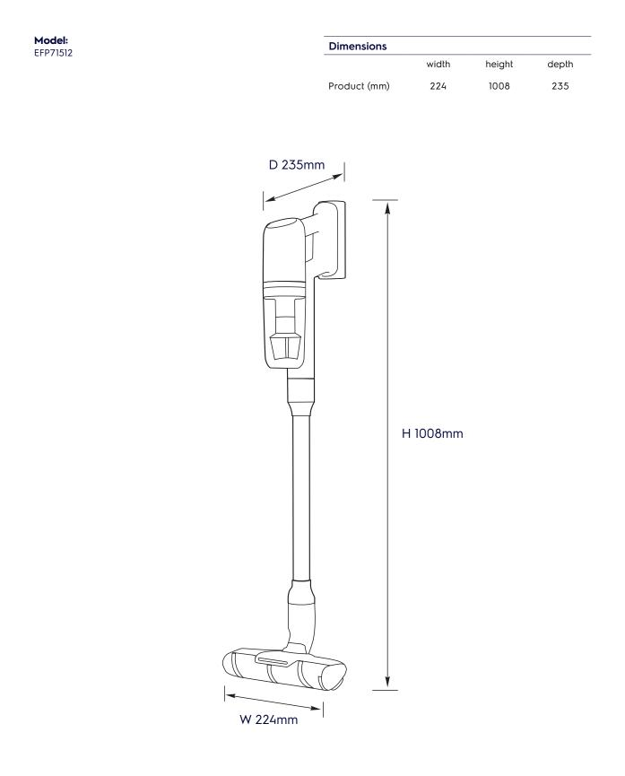
Please note! Dimensions to be used as a guide only. All customers MUST refer to the user manual supplied with the product for detailed installation instructions. © 2022 Electrolux S.E.A PTE. LTD. E\_DIM\_EFP71512\_Apr22
