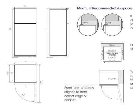
If you do not have a cupboard with allowance for air flow above the refrigerator, the recommended clearance area on top increases to 90mm.
