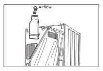
Inlet and outlet points need clear airflow to prevent overheating, so ensure there is adequate ventilation. (i.e. open window or external door.)
