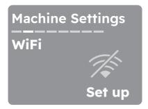
6. Tap the right soft key to set up WiFi connection. The wireless module begins starting up. It may takes about 10 seconds before it is ready.
