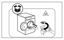
The rear drum locks are removed automatically when the dryer is activated for the first time. Possible to hear some noise.
