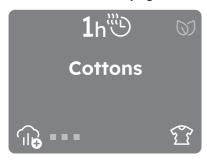
To remove the time drying option, select another programme by rotating the programme dial or reduce the time by pressing the "Time Dry" again and left soft key "" vuntil display to programme time.
