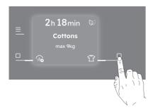
Tap the left soft key "\[ \]" to prompt the action that appears on the left bottom of the display (e.g. & Extra Anticrease, \( \) Final dryness level for Wool programme, \( \) Stem Level, activate or deactivate an option.) the menu,...).
