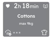
After two seconds, the display will show the selected cycle as a favourite recognizable by a heart "O" at the top of the screen. (i) When you want to save the next favourite the first empty slot will be indicated automatically.
