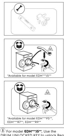
DRUM UNLOCKED KEY to unlock Rear Drum locks, before using the appliance. For other models, the rear drum locks are removed automatically when the dryer is activated for the first time. Possible to hear some noise.
